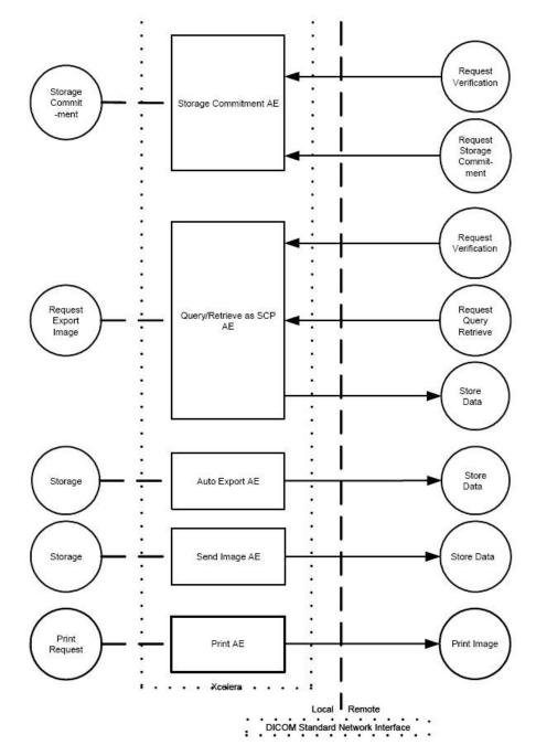
Figure 2: Application Data Flow Diagram (2)
